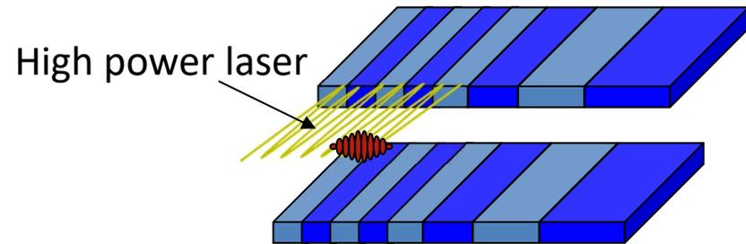
*Undulator magnetic field to couple high power radiation with relativistic electrons*
