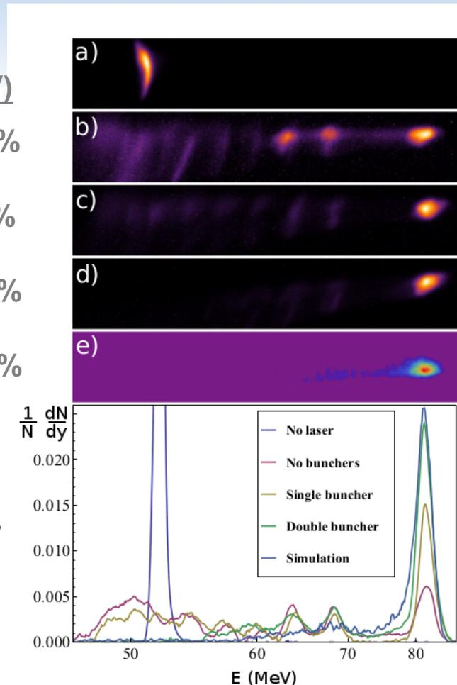
Arxiv: Sudar et al. Demonstration of cascaded modulator-chicane micro-bunching of a relativistic electron beam
