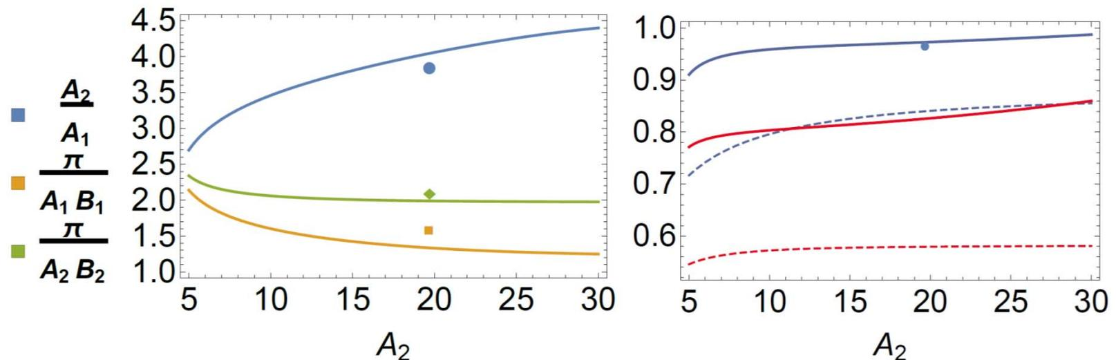
FIG. 2. (left) optimal double buncher parameter values maximizing trapping. (right) Double buncher fraction trapped and bunching factor (blue, dashed) and single buncher fraction trapped and bunching factor (red, dashed). Points at  $A_2 = 20$  are experimental values.
