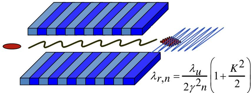
In an IFEL the electron beam absorbs energy from a radiation field.
